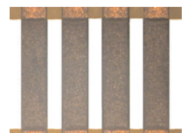
Double-sided exposure of 2 oz. copper fingers on .100" pitch FPC
