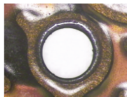
Glue "squeeze out" removal from .050" dia. hole to create 0.010" minimum platable annular ring
