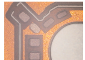
Single-sided exposure and outline of two-layer FPC with .030" x .050" rectangular pads
