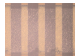
Double-sided exposure of 2 oz. copper fingers on .100" pitch FPC
