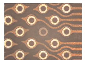
Single-sided exposure and through-holes of a two-layer FPC with .042" dia. exposures on a .100" x .050" through-hole connector pattern
