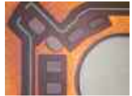
Single-sided exposure and outline of two-layer FPC with .030" x .050" rectangular pads
