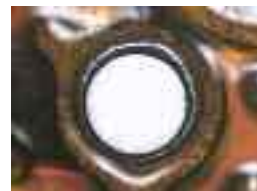
Glue "squeeze out" removal from .050" dia. hole to create 0.010" minimum platable annular ring
