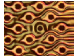
Single-sided exposure and through-holes of a two-layer FPC with .042" dia. exposures on a .100" x .050" through-hole connector pattern
