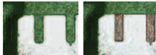
Rework to remove solder mask from a high value rigid-flex
