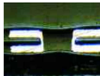
Etched 0.006" vias created in a copper clad laminated by a laser removal of the insulation
